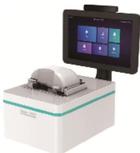
Nano-8000 is a high-throughput full wavelength micro-spectrophotometer that can provide UV/Vis absorbance detection for up to 8 samples in one run. And also has OD600 and single-tube fluorescence detection functions.
